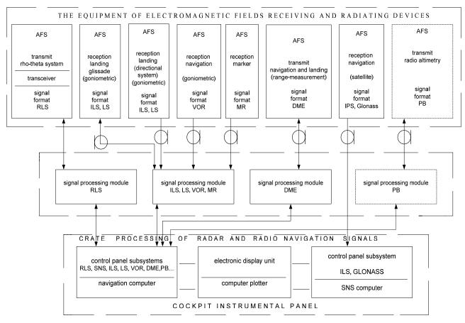
Fig. Structural scheme of radiolocation-navigation-landing complex of aircrafts
