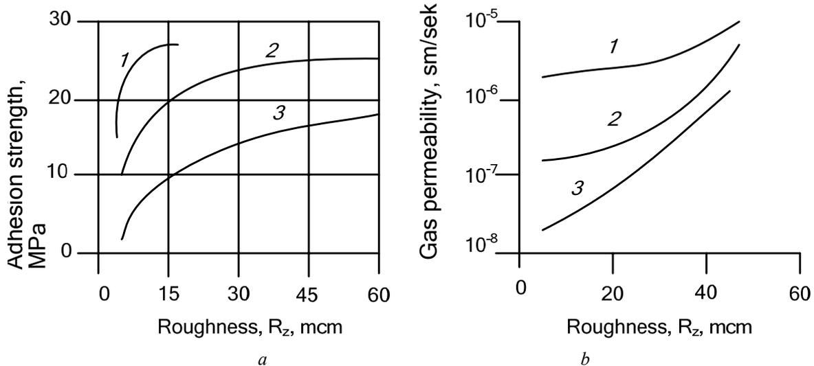
Fig. 3. The effect of the base roughness on (a) the adhesion strength and (b) gas permeability of (1) traditional EAS and (2, 3) activated EAS at a spraying distance of (1, 3) 100 mm and (2) 50 mm
