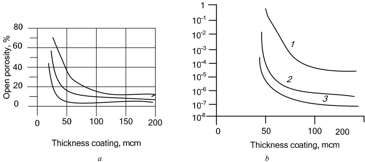
Fig. 2. The effect of the coating thickness on (a) the open porosity and (b) gas permeability: (1) EAS; (2, 3) AAS at a coating thickness of (1, 3) 100 mm and (2) 50 mm
