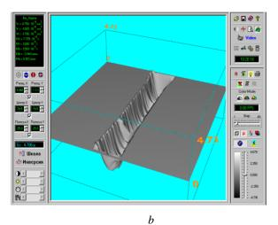
Fig. 3. Profile of track after friction by NANOFOCUS (a) and 3D view of track after friction by DFLSPP (b)
